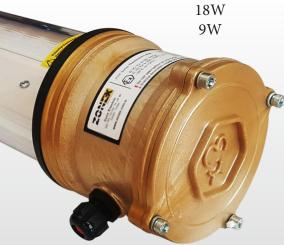
ZNP.X SERIES type fluorescent lamp comprises a lamp tube assembly ith two end caps. The housing consists of a transparent polycarbonateube with polycarbonate end caps. The electronics are located in the main body. Both end caps connected together by two imm diametertie bars, therefore compressing the tube and caps. The equipment is intended for fixed installation. The equipment has normal fluorescent lamp, led fluorescent lamp and emergency kit variations.
